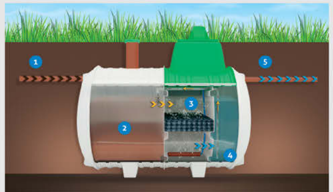
Tricel Novo Wastewater Treatment Plant has an overall efficiency of 95.9% BOD removal
